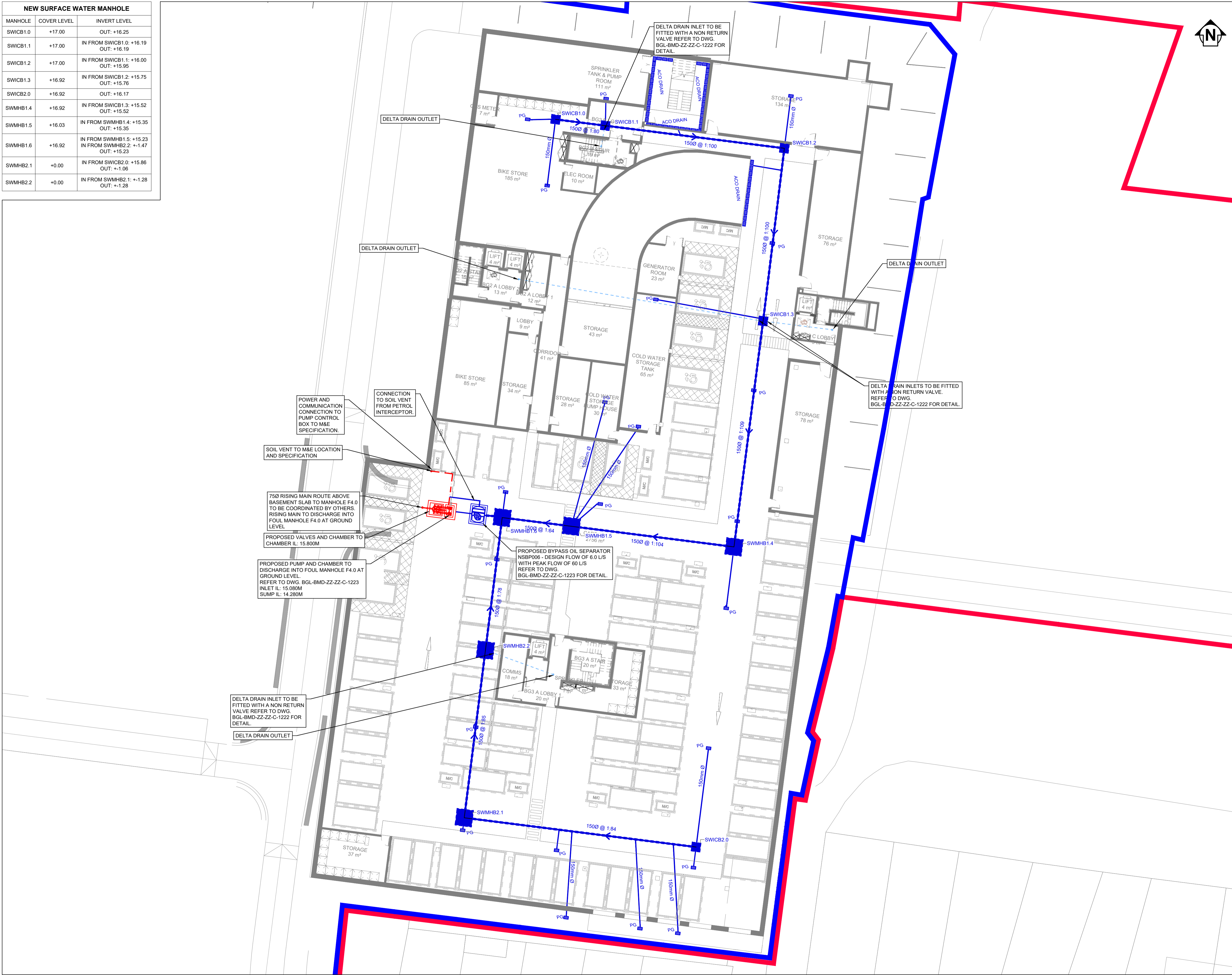
PROPOSED BASEMENT DRAINAGE LAYOUT SCALE @ A1: 1:200 SCALE @ A3: 1:400
